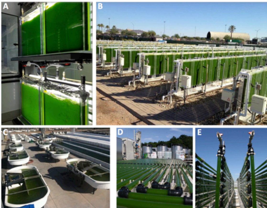
Figure 3-6: Cultivation systems for algae growth. (A-B) flat panel photobioreactors at AzCATI, 39 (C) Small, 1000 L research open ponds at AzCATI, and (D-E) horizontal and vertical tubular photobioreactors at Algae PARC (between 12m 2 and 24 m 2 each) 118
