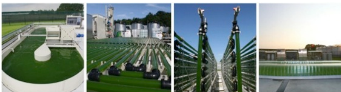
Figure 7-4: The four types of algal cultivation reactor systems being investigated at AlgaePARC installation at Wageningen UR, The Netherlands: (left to right) open raceway pond, horizontal tubular PBR reactor, vertical stacked tubular PBR reactor and flat panel PBR reactor).
