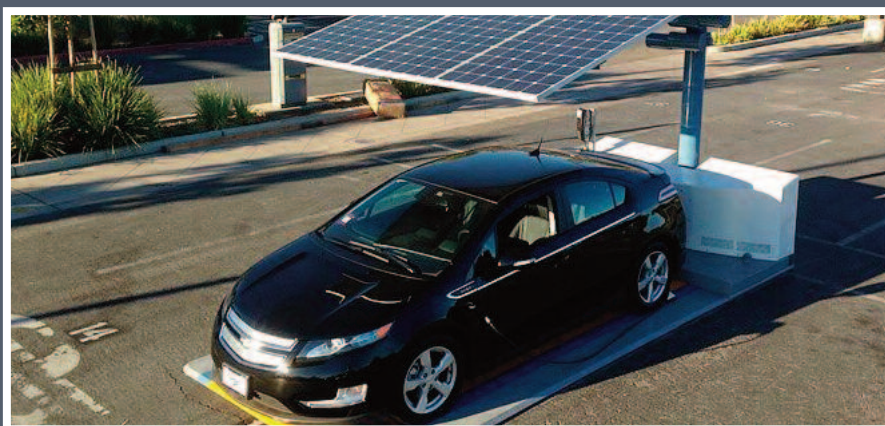
Envision Solar's EV ARC is the first portable solar charging station for electric vehicles
