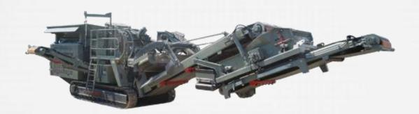
The new Rockster R1100DE full hybrid stone crusher using full Visedo electric drive train is now released to sales with first delivery to major French road construction company. The Rockster hybrid crusher is the first of it's kind in the market and the innovative machine brings 16 000 liters of annual diesel savings and at the same time increases the crusher productivity."
